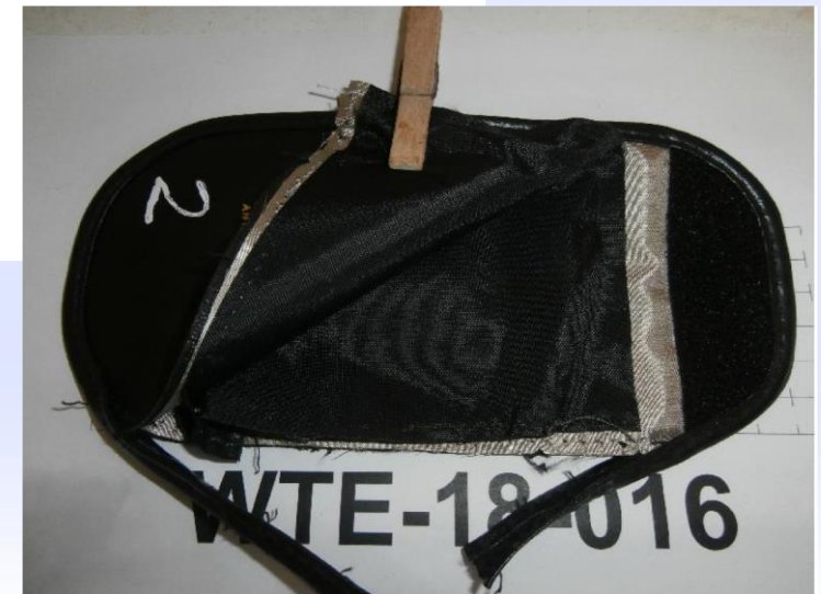
Key Pouch at Completion of Test (20,000 cycles)
